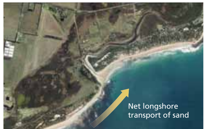
Figure 44 Headland reduces sand build-up (Thompson Creek Estuary)
