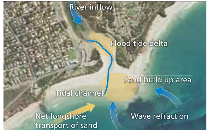
Figure 43 Offshore reef exacerbates sand build-up (Anglesea River Estuary)
