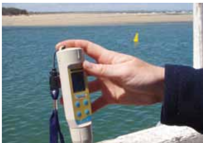
Figure 28 EstuaryWatch monitor using the PCS Testr 35 Meter to test for pH
