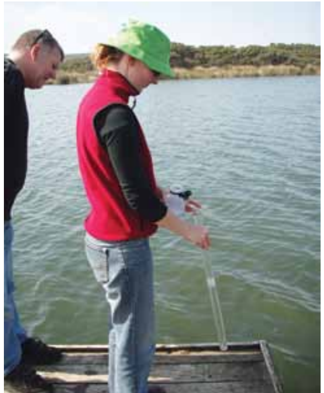
Figure 26 Turbidity monitoring at Anglesea River Estuary
