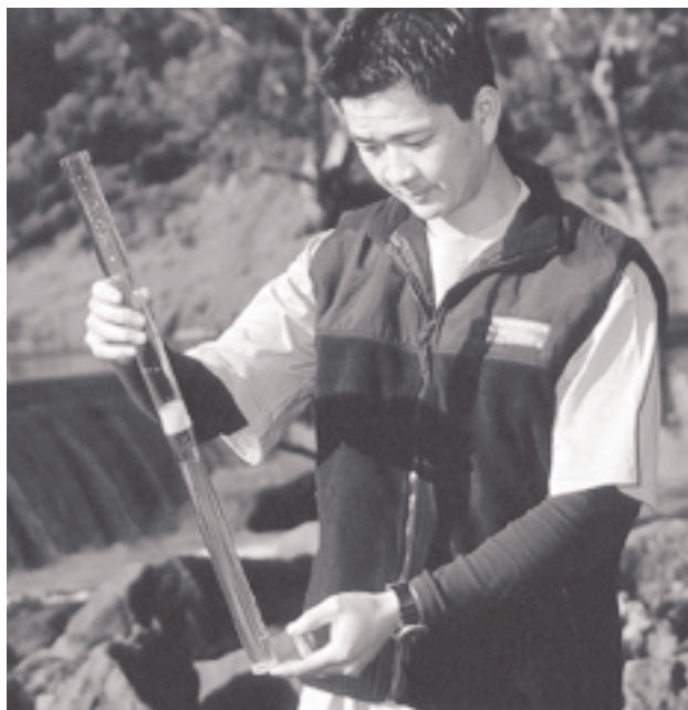
Paulo Lay from the Department of Sustainability and Environment demonstrates how to read turbidity tube.
